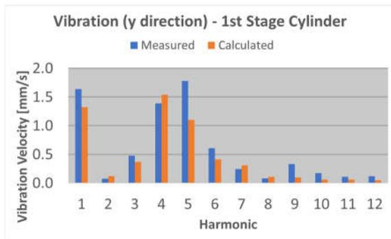
Figure 19: 1<sup>st</sup> stage cylinder vibration in vertical direction (y)
