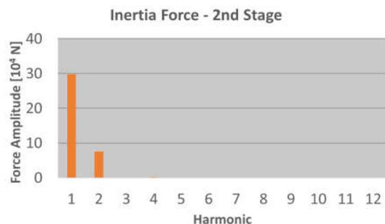
Figure 10: 2<sup>nd</sup> stage inertia dynamic loads
