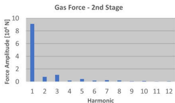
Figure 9: 2<sup>nd</sup> stage cylinder gas dynamic loads
