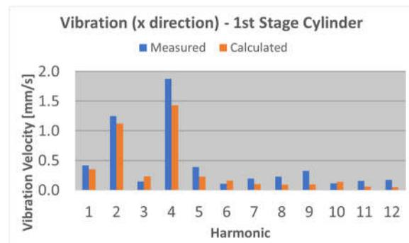
Figure 18: 1<sup>st</sup> stage cylinder vibration in compressor shaft axis direction (x)
