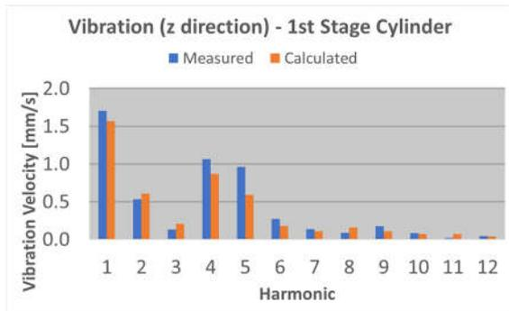
Figure 20: 1<sup>st</sup> stage cylinder vibration in cylinder axis direction (z)
