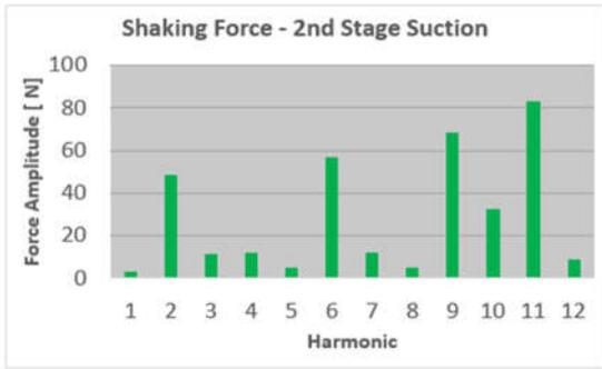
Figure 11: 2<sup>nd</sup> Stage Suction Damper shaking forces
