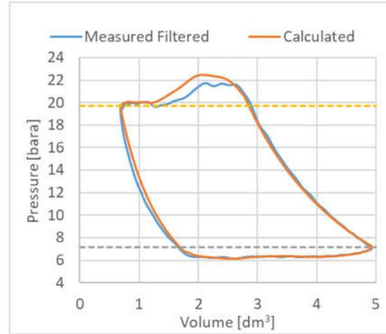
Figure 13: PV-cycle 2nd Stage Cylinder CE – measured filtered vs. calculated
