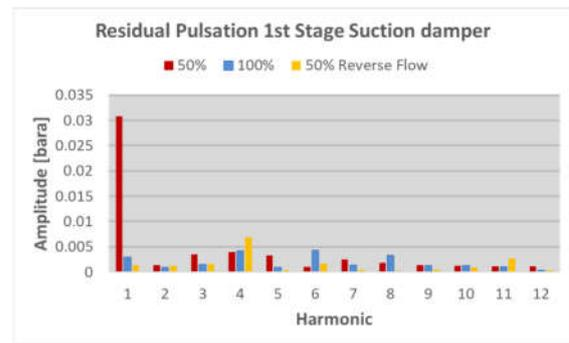
Figure 21: Residual Pulsation @ 1<sup>o</sup> Stage Suction Damper Nozzle line side
