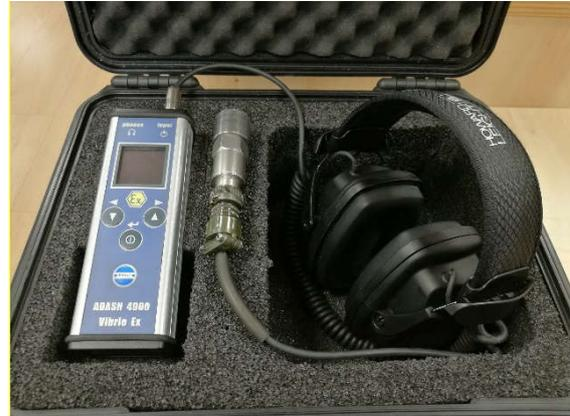
Figure 3: Accelerometer for vibration diagnostic
