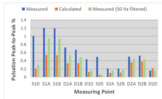
Figure 14: Pulsation amplitude in the measuring points: 6th Harmonic
