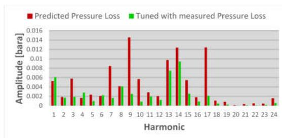
Figure 16: Effect of heat exchanger model on pulsation
